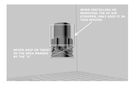
Because of the multiport forward end, it will not be able to withstand high amounts of torque or lateral forces. When removing your barrel shroud turn the shroud as you remove it and never cock or bend the shroud which will apply undue stress on the air stripper and break it. Be sure to apply silicone lube to the inside of the shroud and o-rings to assist in the installation.
